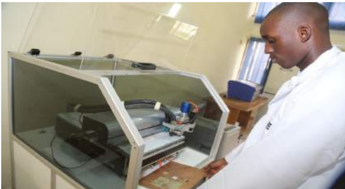
Figure 6: Printed Circuit Board Machine in the Digital System and Prototyping (Printed Circuit Board) Laboratory
